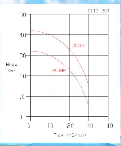
The main features of our heavy duty slurry pump is a heavy design of wear resistant casing and 28% HiCr impeller. Excellent combination of materials provides long term operation even in harsh abrasive slurries.
